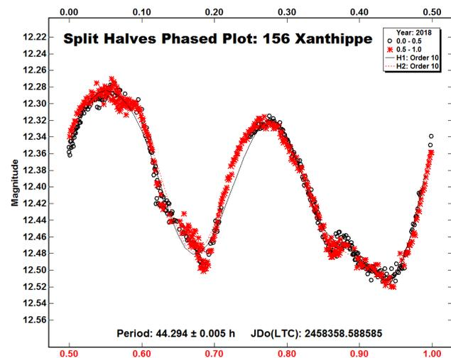
Figure 2. Split halves lightcurve of 156 Xanthippe phased to the double period 44.294 hours.
